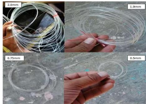
Figure 3.4: Plastic optical fibers used in this project.
