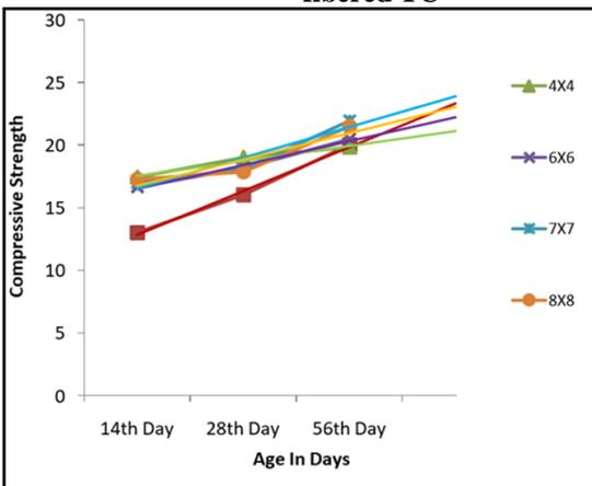
Figure 4.6: Compressive strength for 1.0mm diameter fibered TC
