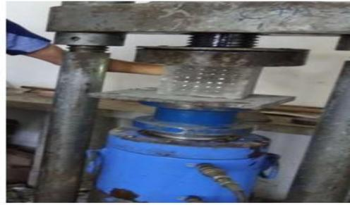
Figure 4.3: Translucent concrete cubes under compressive strength testing.
