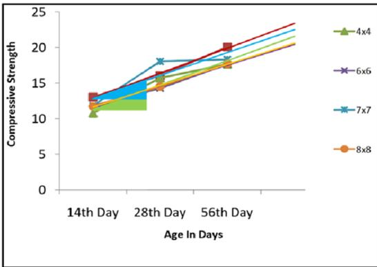
Fig 4.5 . Compressive strength for 0.75mm diameter fibered TC
