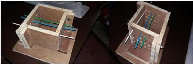
Fig 3.6. Wooden moulds for casting of translucent concrete.
