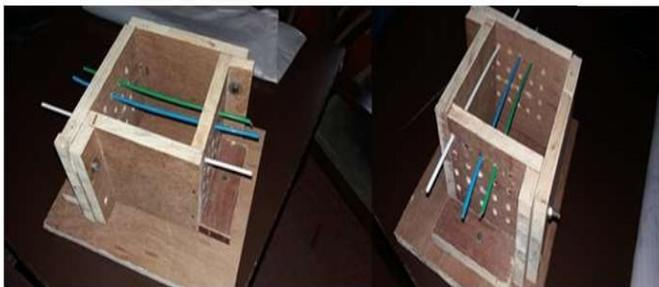
Fig 3.6. Wooden moulds for casting of translucent concrete.
