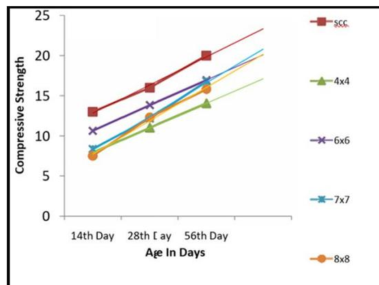
Fig 4.4. Compressive strength of 0.5 mm diameter fibered TC
