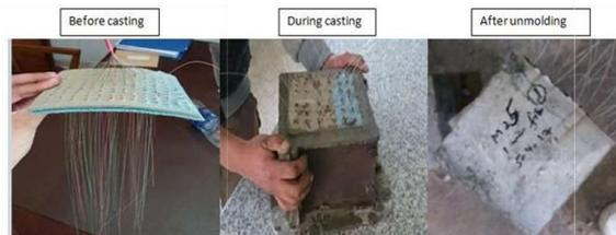
Figure 3.5: Card board holding optical fibers to be inserted in
